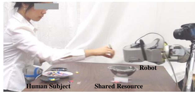
Figure 1. Experimental setup for our in-situ HRI study. A participant performs a task where there is a frequent need to access the resource shared with the robot.
